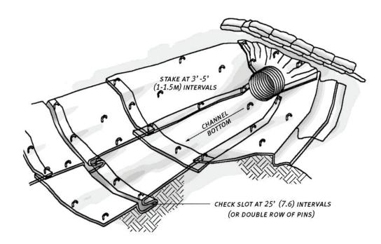
1.5" x 12" metal pins, 8" - 18" pins with 1.5" diameter washer, or 12-30"-J Shapepins (bent rebar) having a ¼" diameter. Drive pins or pins flush with the ground surface.
